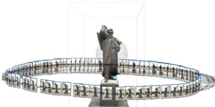
Figure 2. Generated 3D textured model of the Svetozar Miletić monument (by the photogrammetry) in AgiSoft Metashape.
