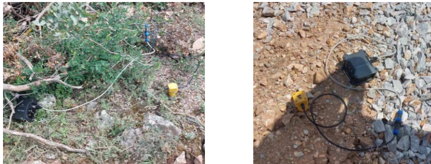
Figure 2. ZOOM F6 connected with one vertical geophone.
