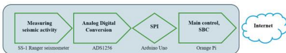
Figure 2. DAQ system general block diagram.
