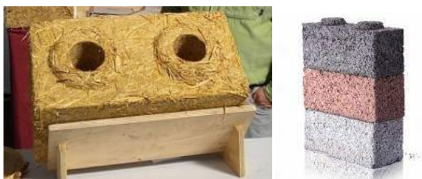
Figure 7. Compressed straw blocks in the Lego design (Wilson 2009).
