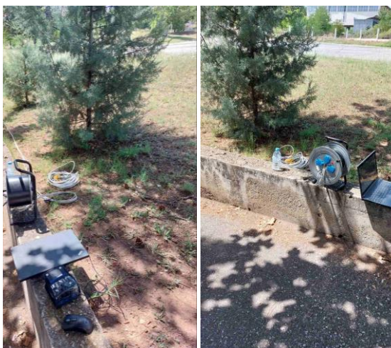
Figure 4. Application of multistring system of geophones connected to ZOOM's (induced seismic from seismic hammer).
