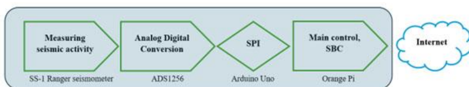
Figure 2. DAQ system general block diagram.
