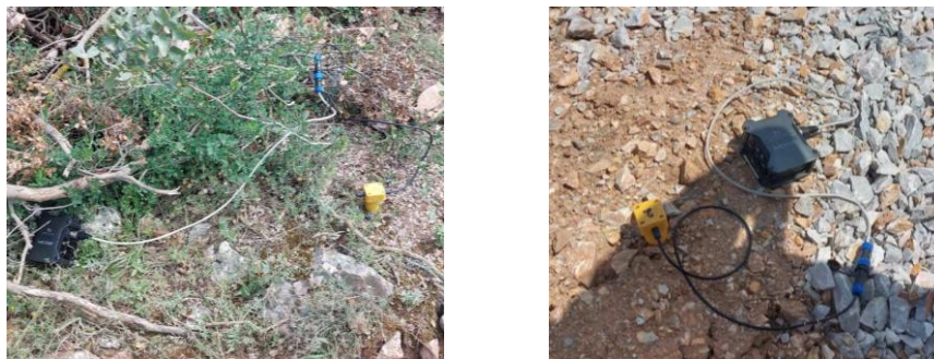
Figure 2. ZOOM F6 connected with one vertical geophone.
