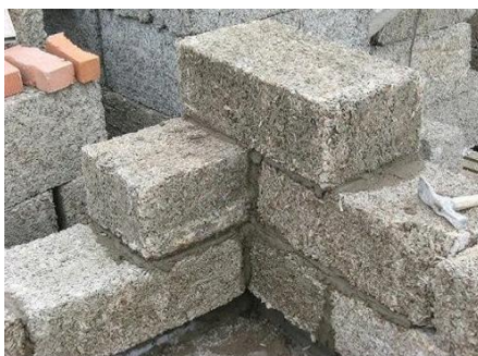
Figure 8. Straw concrete blocks (sand and gravel+ cement+straw).
