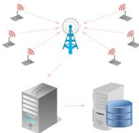
Slika 3 IoT arhitektura (senzori, bazna stanica, mrežni server, aplikativni server)(S.Salapura, 2019) Figure 3 IoT architecture (sensors, gateway, network server, app server) (S.Salapura, 2019)
