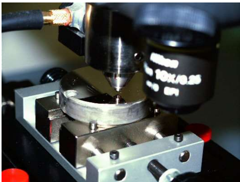
Figure 6 Close up to adhesion testing of the cylindrical sample after coating deposition
