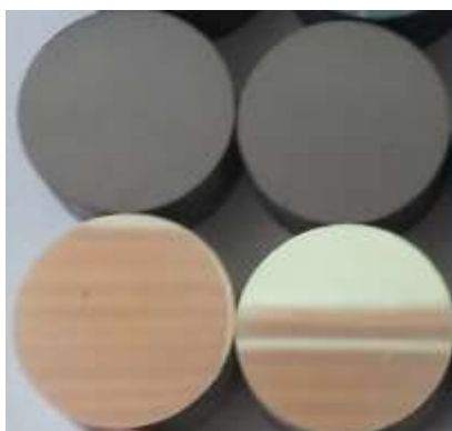
Figure 1 Samples of high-speed steel after coating deposition
