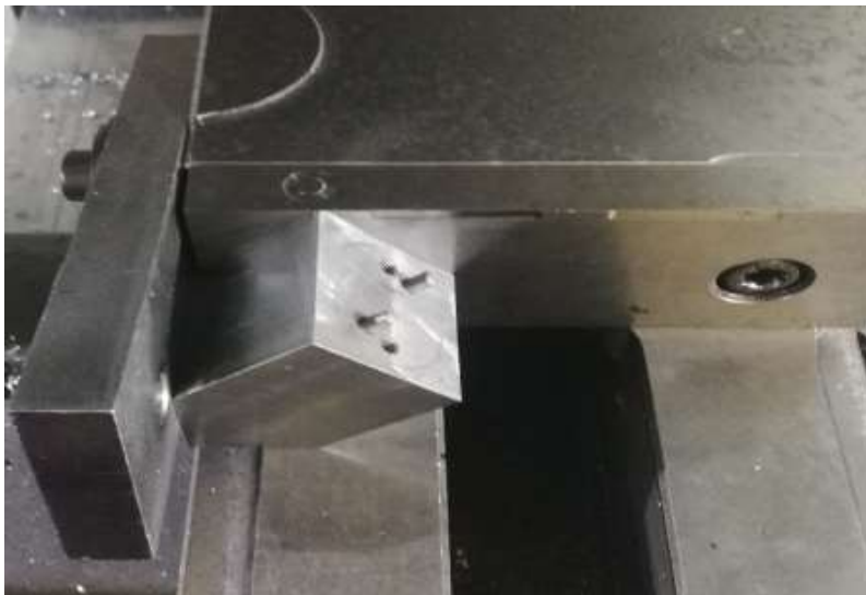
Figure 7. Jig implemented to the production process
