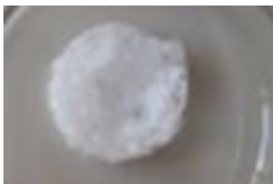
Figure 1. Xerogel obtained in microwave field.
