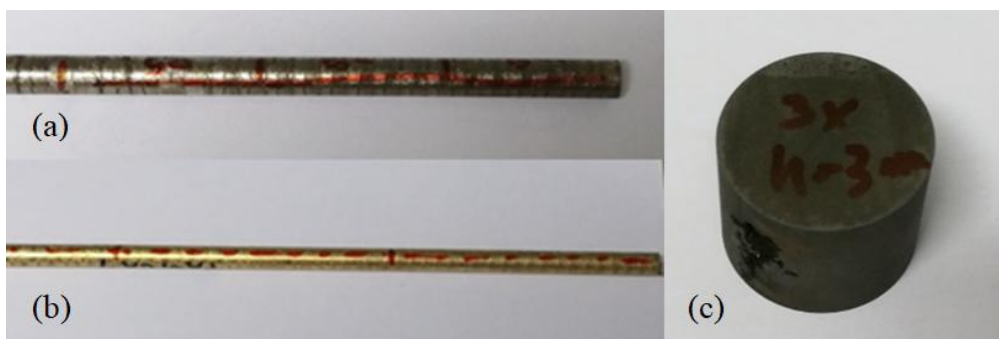
Slika 1. Ni-Ti CC (a), Cu-Al-Ni (b) i Ni-Ti as cast (c) (Ivošević, Vastag, Majerić, Kovač i Rudolf, 2020). Figure 1. Ni-Ti CC (a), Cu-Al-Ni (b) and Ni-Ti as cast (c) (Ivošević, Vastag, Majerić, Kovač, & Rudolf, 2020).
