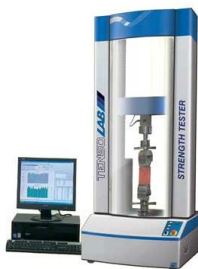
Figure 1. MESDAN-LAB tensile Strength Tester (TENSO-LAB).
