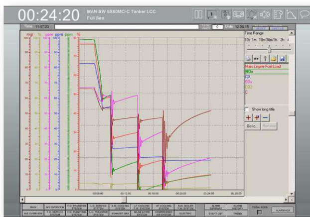
Figure 2. Diagram which shows the decrease in speed and emission of negative gases in a period of 30 minutes.
