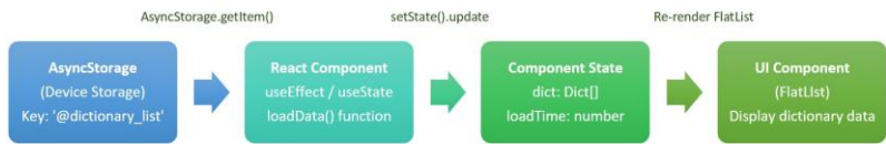
Figure 3. Data flow: AsyncStorage → Screen (React Native).
